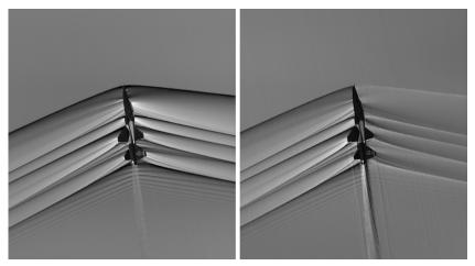
Left: Schlieren image dramatically displays the shock wave of a supersonic jet flying over the Mojave Desert. Averaging multiple frames produce a low-noise picture of the shock waves.
