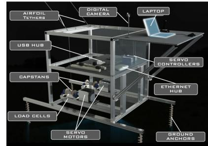
Ground station for NASA Langley wind energy prototype
