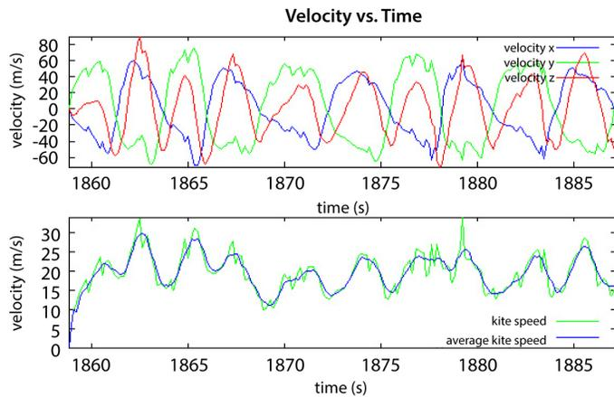
Auto-Pilot Flight Testing Velocity from Visual Tracking
