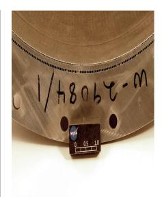
Interim inspection improves the quality of parts with intricate internal features like these fuel channels.
