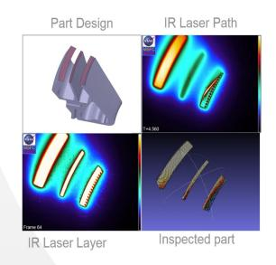
The NASA technology can be used to determine geometric differences (flaws) between the designed model and the printed part/component.
