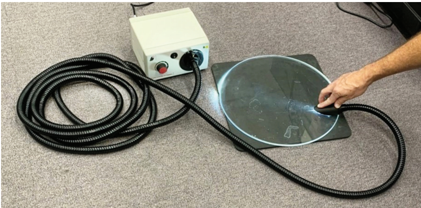
The delivered SLOT using a 20-foot length of multimode fiber and remote light supply.
