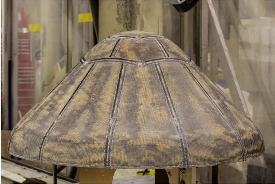
Fig. 5 Full scale (1 m diameter) integrated engineering test unit (ETU). The nose tile, two rows of circumferential tiles, circumferential and radial seams between the acreage tiles and closeout plugs are all integrated to form the heatshield
