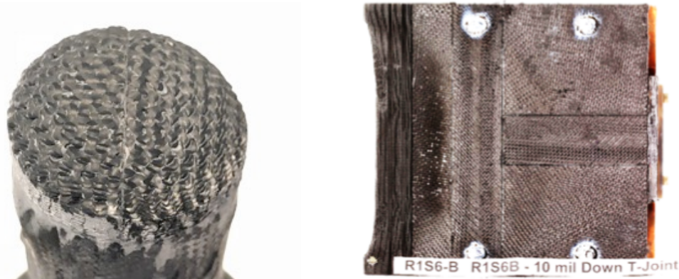
Figure 3. (Left) Post-test IHF stagnation model showing successful test of 0.25mm thin Nitrile Phenolic adhesive seam , (Right) post-test AEDC wedge model showing successful test of a T-Joint.
