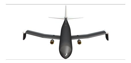
A rendering of an aircraft equipped with SAWs, wherein the wingtips are folded downwards. Outer ailerons are placed on the wingtips, and are driven by NASA's novel control algorithms to achieve desired yaw and roll accelerations.
