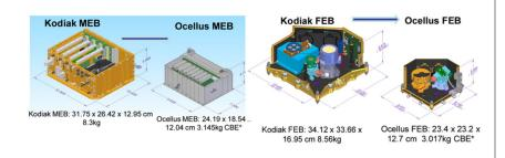
Images showing the design and development of the Ocellus that is based on the previous Kodiak 3D lidar system (MEB = main electronics box, FEB = frontend box).
