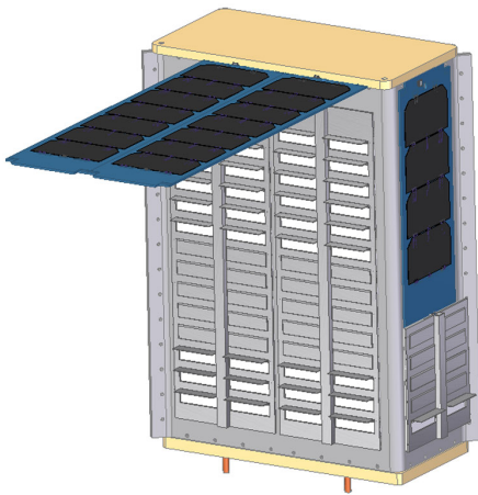
CubeSat Form Factor Thermal Control Louvers on a 6U CubeSat
