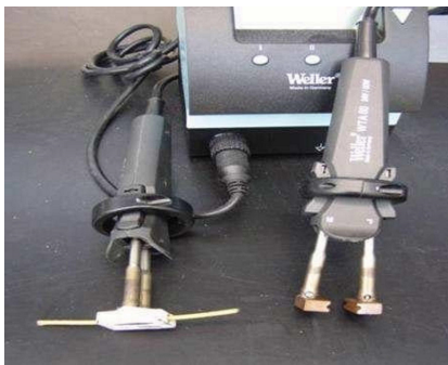
Wire Repair Heating Tools
