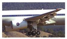
Invention is best applicable with pylon downstream of the exit plane of the core nozzle exit (as pictured).
