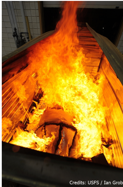
Fire shelter under test conditions.
