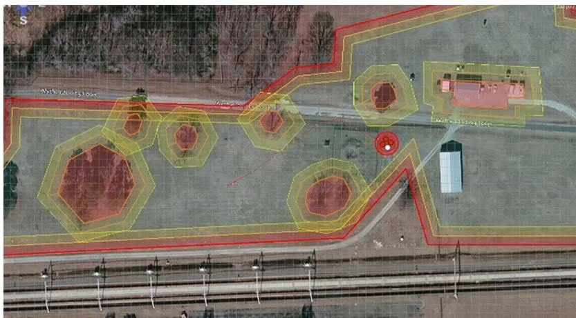
Ground station display of containment system boundaries during flight. Image source: NASA
