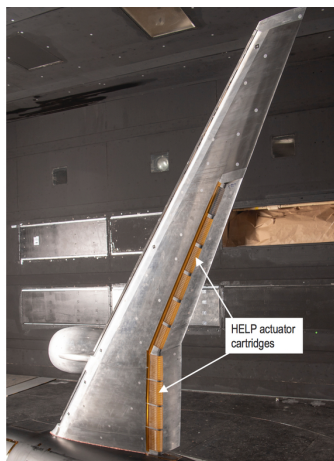
HELP actuator cartridges on the NASA High-Lift Common Research Model (CRM-HL). Testing proved that HELP flow control actuators were very effective in controlling the substantial flow separation on a simple-hinged flap system with a 50 degree flap deflection.
