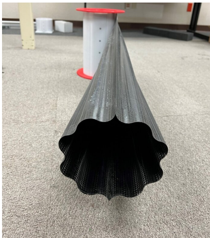
COROTUB reaches its full extension over a shorter distance compared to non-corrugated boom designs.
