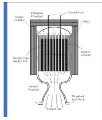
Shown is the design for NTAC Augmented Nuclear Electric Propulsion and/or Nuclear Thermal Propulsion. The the NTAC Augmented Nuclear Electric NTAC surrounds the rocket chamber on Propulsion and/or Nuclear Thermal all sides and the topmost portion.
