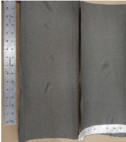
Image of Ta/Ti glass fiber fabric samples.
