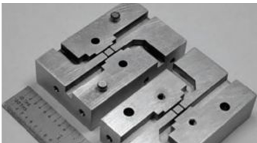
Glenn's technology combines unequal output powers, permitting more flexibility in space communications system design
