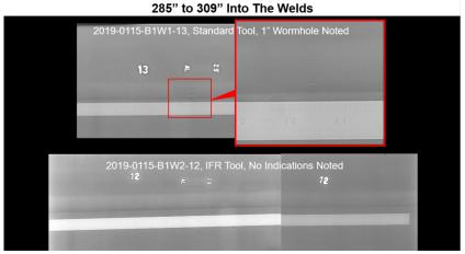
Weld inspection x-rays show a defect 300" into a SR-FSW weld made with a standard pin tool (top image). No defects were found in the first 900" of an IFR Tool weldment (bottom image).
