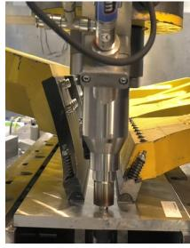
The IFR Tool–shown performing a SR-FSW panel weld in the image above–enables a more robust and thereby cost-effective SR-FSW process.
