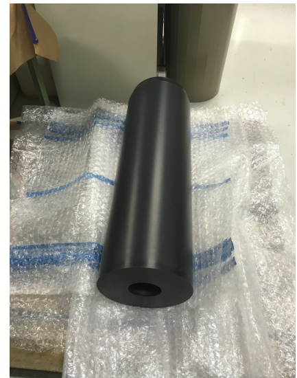
A monolithic paraffin fuel grain cast with the novel oven cooling process and devoid of cracks. The paraffin fuel grain is full-scale for use in Mars Ascent Vehicles.
