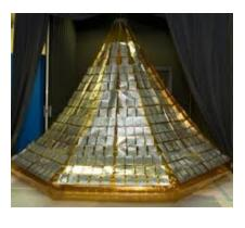
NASA's lightweight, self-deployable helical antenna will be integrated into the Lightweight Integrated Solar Array and Transceiver (LISA-T) - a launch stowed, orbit-deployed array on which thin-film photovoltaic and antenna elements are embedded.
