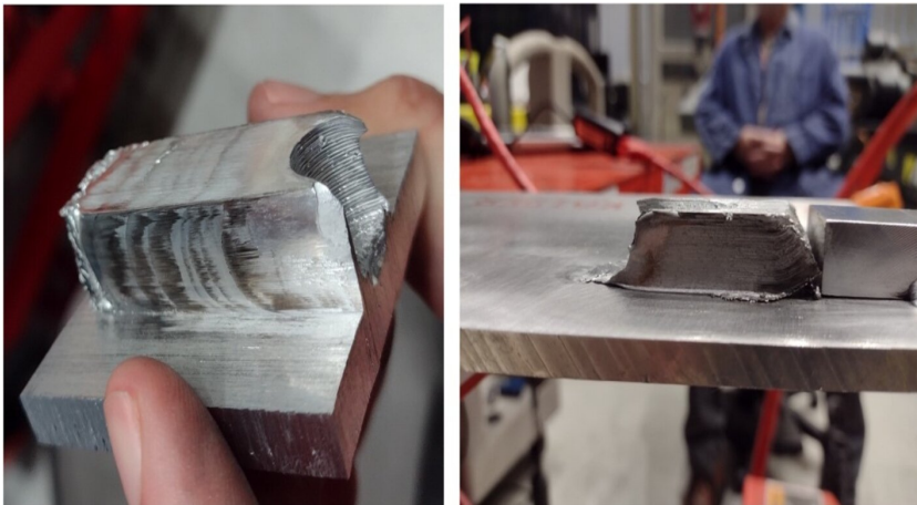
Demonstration articles of the additive friction stir deposition processes.
