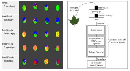
Hyperspectral images captured for leaves dosed with TCE over varying time periods; these are examples of response Diagram of the hyperspectral estimator signatures to be built into the device's reference library/database
