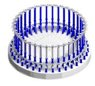
NASA's tooling is made of individual components that are selected, assembled, and adjusted depending on the size and shape of a finished part. CAD models are easily reproduced on the production floor using the modular tooling.
