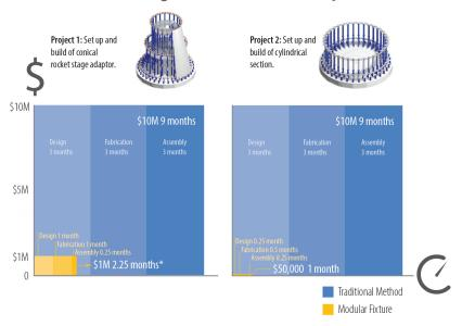
This graphic illustrates how NASA's development of modular fixtures significantly reduced its costs for designing, fabricating, and assembling welding tooling. \*Project 1's cost of \$1 million when using the modular fixture method includes the cost for the initial development of the modular fixture platform. Reuse of the modular fixtures results in future cost savings in subsequent projects.
