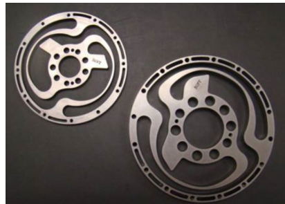
Custom torsion springs (U.S. Patent No. 8,176,809) from the R2 series elastic actuators.
