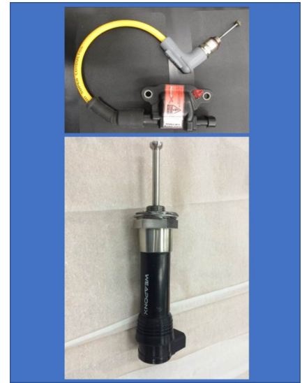
Top: Conventional spark plug with external coil and high voltage-cable. Bottom: Coil-on-plug spark plug system with high voltage cable eliminated.
