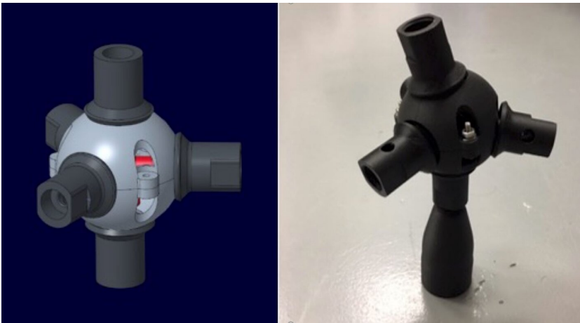
Shown (left): CAD Design and (right) 3D-printed prototype of the Multi-Link Spherical Joint.
