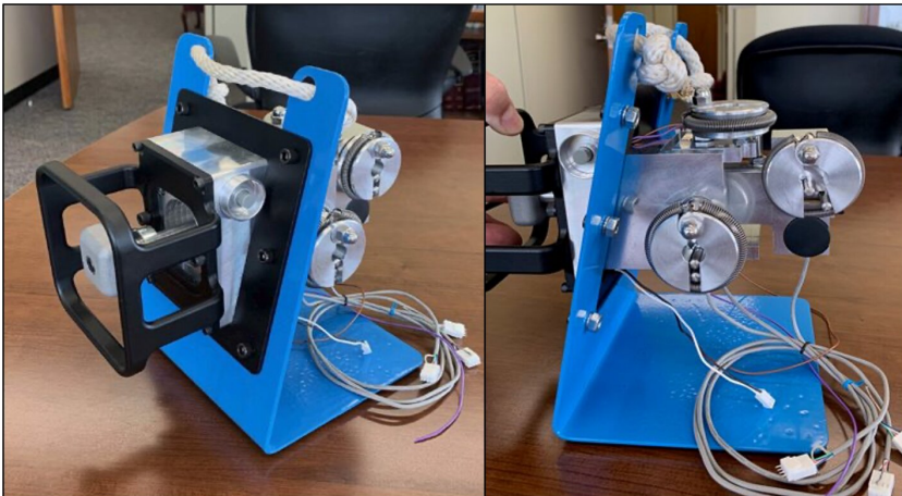
Shown: Three-quarter view of three-axis analog hand controller (left) engineered with Circumferential Scissor Springs, and side view of controller (right) with control stick being pushed inward, initiating circumferential spring return-tension.
