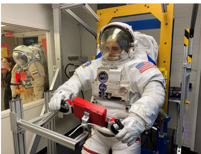
Shown: A suited astronaut tests the user interface of a Tri-Rotor steering wheel prototype
