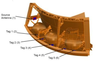
The antenna and distributed sensor tags stream low-rate thermocouple data from a heatshield. In hybrid sleep/wake mode, sensors run for 5+ years on a CR2032 coin cell battery; in active state, they stream 10 Hz data for 200+ days.
