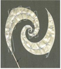
prototype comprised of Nora Dell conductive fabric, a polyester fabric substrate, and RG178 coaxial cable.
