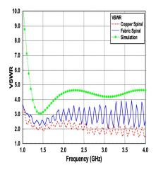
Fabric spiral antennas using this method Shown is a fabric-based spiral antenna performed similarly to conventional copper antennas across multiple metrics, including VSWR.
