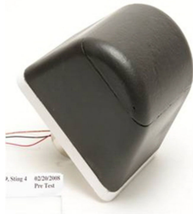
Toughened Uni-Fibrous Reinforced Oxidation-resistant Composite (TUFROC)
